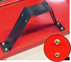
Attach the drawbar bracket to the bottom of the cart with 4x x-head bolts.
