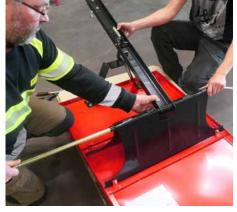
Attach the axle and the drawbar as shown in the picture.
