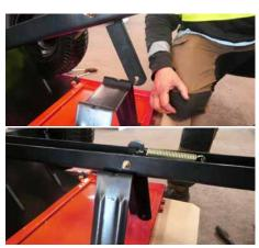
The drawbar is locked in the drawbar bracket.
