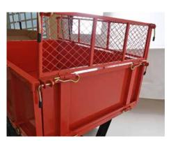
Attach the mesh sides to the cart and fasten them with spring locking pins.
