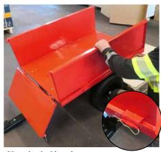
Attach the tailboard as shown in the picture. Clasp the top as shown in the little picture.
