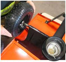
Put the wheels on the axle, add the washers and fasten with the split pins (one on each side).
