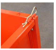
Fasten the tailboard with the spring locking pins with chain.
