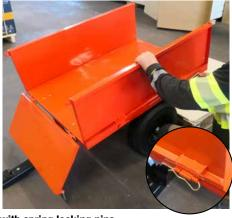
Attach the rails for the tailboard with 4x M6 bolts with x-head.
