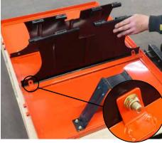
Insert the wheel plates and fasten them with 2x M8 bolts with hex head in each plate. Use 2x 13mm spanners when you screw them in.
