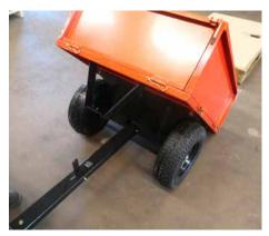
Tilt the cart by pulling the spring loaded locking mechanism.
