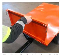
Attach the frontboard and the sides and lock them with spring locking pins.
